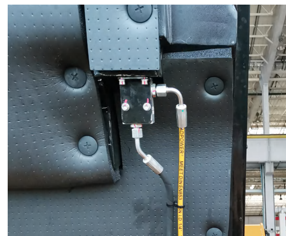
EMERGENCY UNLOADING: Lower the boom in emergency situations to ensure safety.
