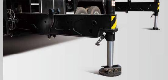
Outriggers extend to 7.7m in full span, making lifting operation more stable. Newly developed half extension mechanism makes the crane more adaptable to work at constricted area.
