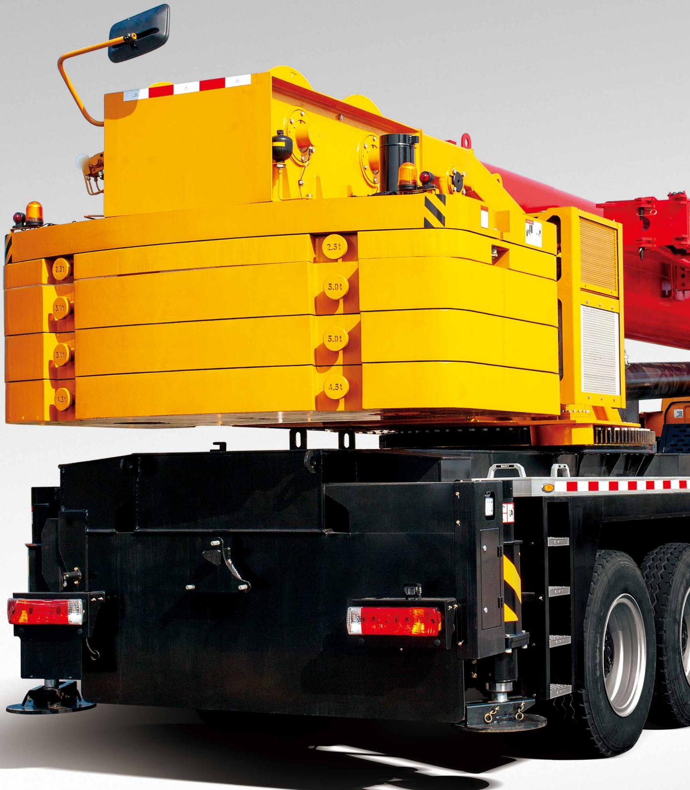
Remark :this illustration is crane with 20t counterweight (optional) in working status, not for traveling.
