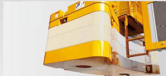
Fixed CW 3t, movable CW 7t, featuring three combinations. Additional 5t or 5t\*2 CW for option. The crane can travel with 15t CW on board at low speed (<20km/h) in short distance. CW assembly efficiency significantly increased via auto-lock after CW lifted to position.
