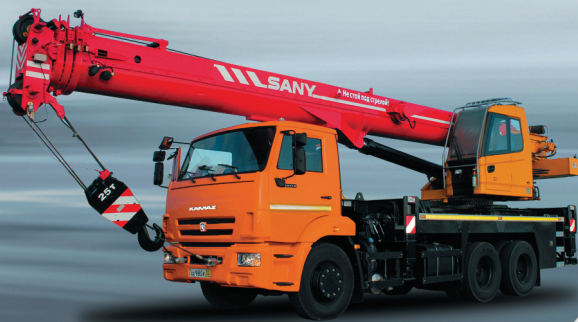
32 TONS TRUCK CRANE BOOM 10.2-32 m
