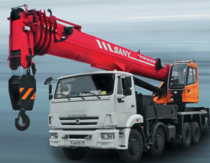
40 TONS TRUCK CRANE BOOM 10.5-49.51 m
