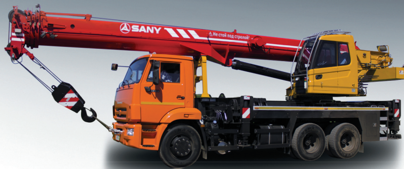
25 TONS TRUCK CRANE BOOM 10.2-32 m
