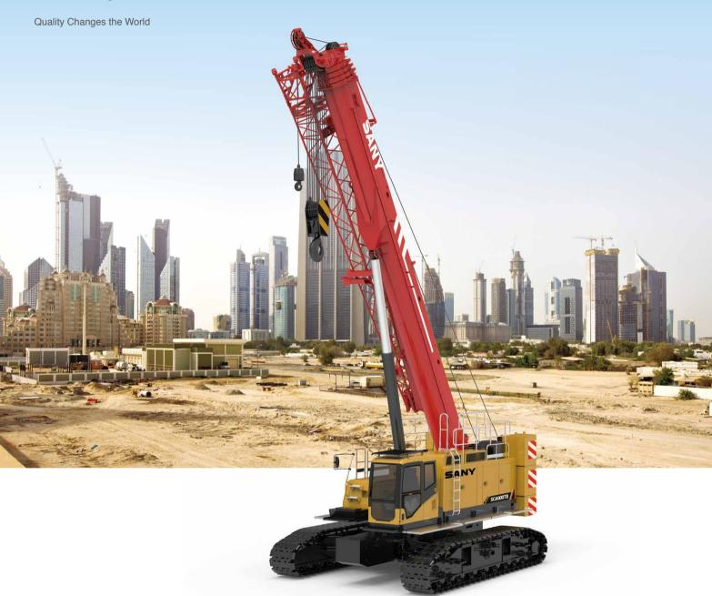
Max. Lifting Capacity: 90 USt Max. Boom Length: 154.2 ft
